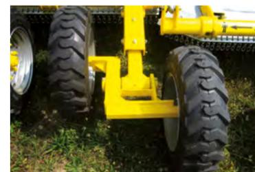
A central swinging axle helps to overcome uneven surfaces whilst maintaining working height. Thanks to the axle the machine is able to operate smoothly even on extremely rough fields and pastures.
