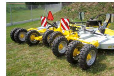
The MM 7000 rotary cutter comes as a standard 8 wheel model. The MZ rotary cutter comes in a standard 6 wheel model but can also be customised to come in an 8 wheel version. The wheels can be filled with foam to prevent puncture.
