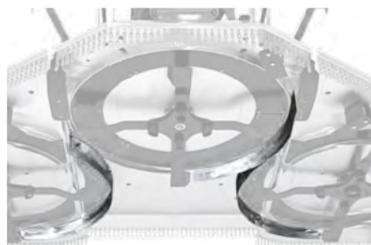
Perfect machine work is ensured by plates that evenly spread the mulched material over the field. Vegetal clusters are not formed, etc.
