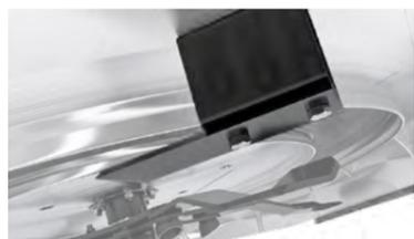
To increase the crumbling effect of the front parts of the mulching zone, they have been equipped with counter blades that complete the cutting of the mulched material. The quality of the mulched material is therefore increased.
