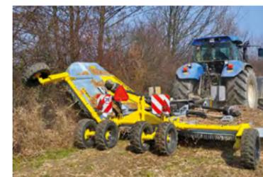
The wings of the MZ and the MM rotary cutters work on a swinging arm and perfectly track unevenness of mulched fields from -15° to +45°. The machine can be used with the side positioned at +45° therefore can be used to clean road sides and along the edges of pastures and fields.
