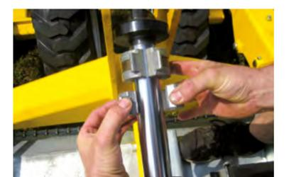
The mulching height of the MZ and the MM machine is set centrally with the help of hydro clips on the hydraulic cylinder conduit of the machine's central axle. Adjustment of the setting is done swiftly and with ease.
